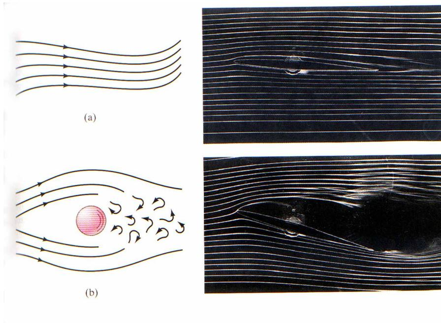
Fig. 1 (a) Streamline or laminar flow; (b) turbulent flow.
