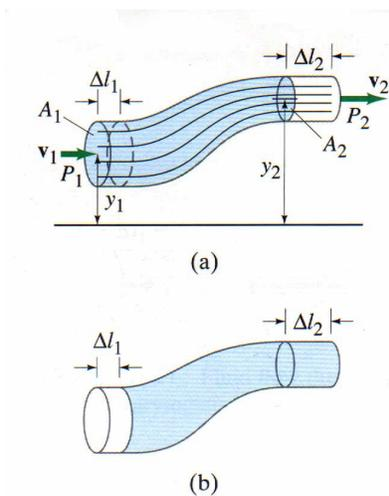
Fig. 6.3 Fluid flow: for derivation of Bernoulli's equation.
