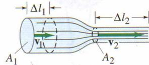
Fig. 6.2. Fluid flow through a pipe of varying diameter.
